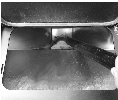
Fig. 24 - Hopper and auger cleaning
