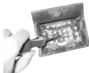
Fig. 21 - Burning pot cleaning
