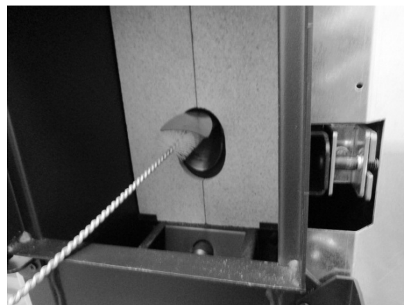
Fig. 23 - Cleaning with a brush
